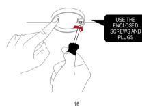
Once the mounting base is installed, attach the alarm by twisting clockwise until it clicks. If the battery is either missing or inserted incorrectly, or the switch is in 'Learn Mode', the heat alarm will not be able to click into
