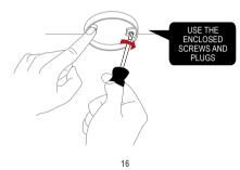
Once the mounting base is installed, attach the alarm by twisting clockwise until it clicks. If the battery is either missing or inserted incorrectly, or the switch is in 'Learn Mode', the smoke alarm will not be able to click into the mounting base.
